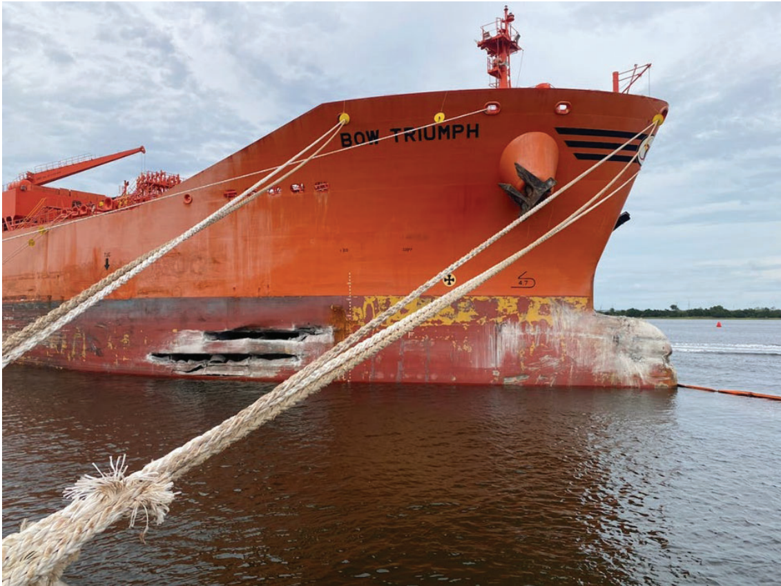
Figure 5 BOW TRIUMPH's damaged starboard bow while moored at Odjell Terminal in North Charleston on 08 September 2022. Photo: U.S. Coast Guard.
